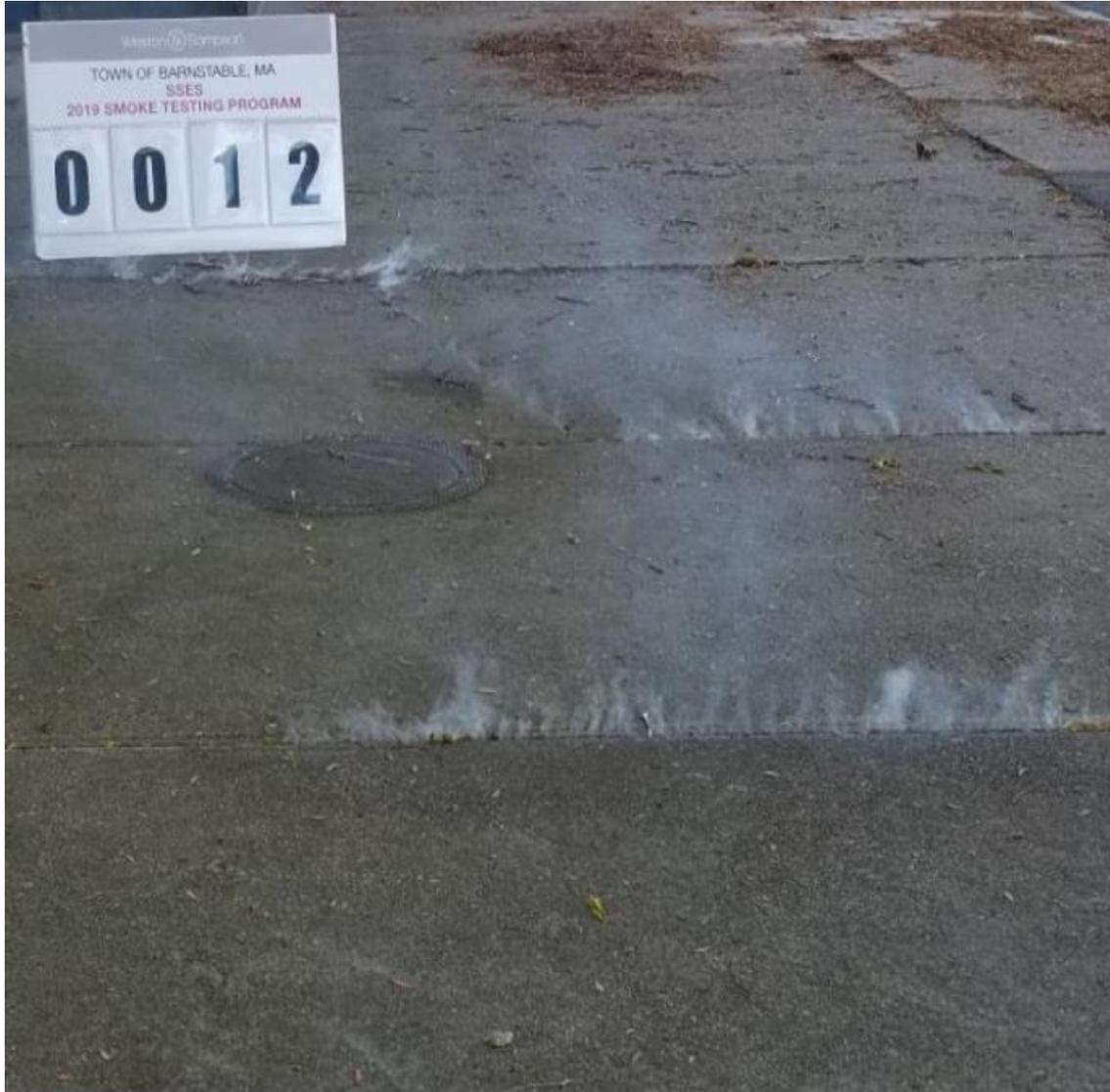
Smoke testing involves blowing smoke into the sewer system to help locate sewer defects. This photo shows an area where smoke is escaping from the sidewalk during smoke testing, indicating that a pipe defect exists in this area.
