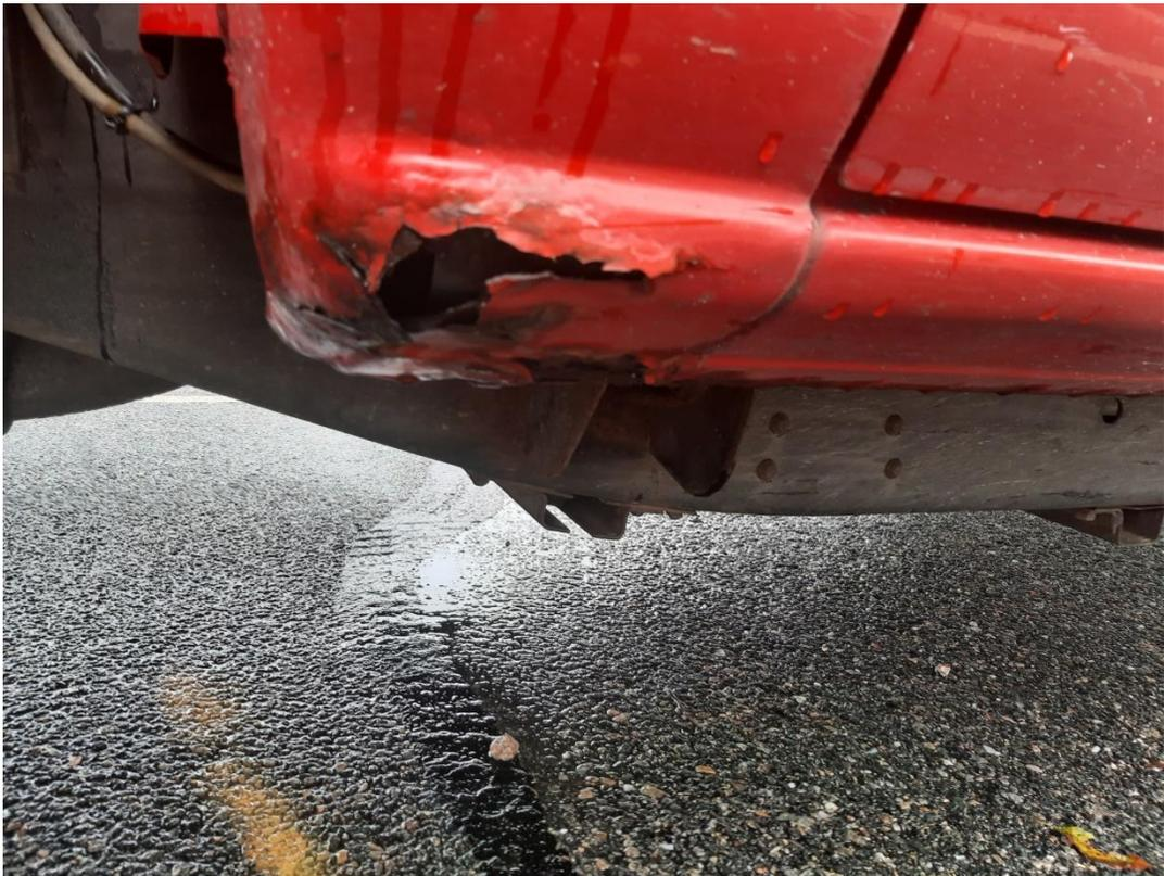
Example of corrosion on Truck 254
